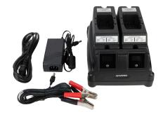
The RF-5853-CH2XX Lithium Ion Battery Charger is used to charge high capacity 12041-2200-XX, 12041-2400-XX and 12500-2500-XX lithium ion battery packs for Falcon® handheld radios. These chargers are available in one-, two- and six-bay configurations. They support power input from AC and DC sources and, in addition to battery conditioning support, can recover a unit which has been overcharged.
