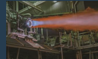
RL10C-X | Additively manufactured RL10 with improved performance
