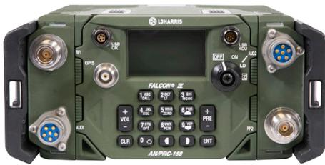
Equipped with a Software Communications Architecture (SCA) and a broad portfolio of narrowband, wideband and fast-hop resilient waveforms, the AN/PRC-158 ensures continuous communications, advanced interoperability and is software upgradeable for new capabilities. The manpack's two channels and superior routing and crossbanding technologies support communications redundancy and critical voice and data sharing with a variety of nets.
