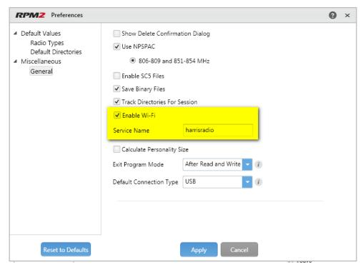
Figure A-4: Enable Wi-Fi in RPM2
