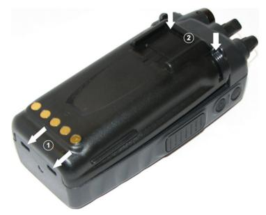
Figure 3-1: Attaching the Battery
