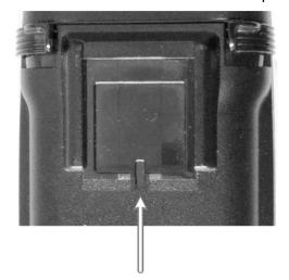
2. Slide the D-Ring out of the slot on the battery.
