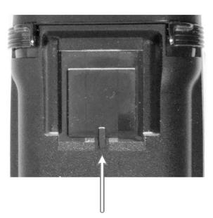
3. Slide the belt clip out of the slot on the battery.
