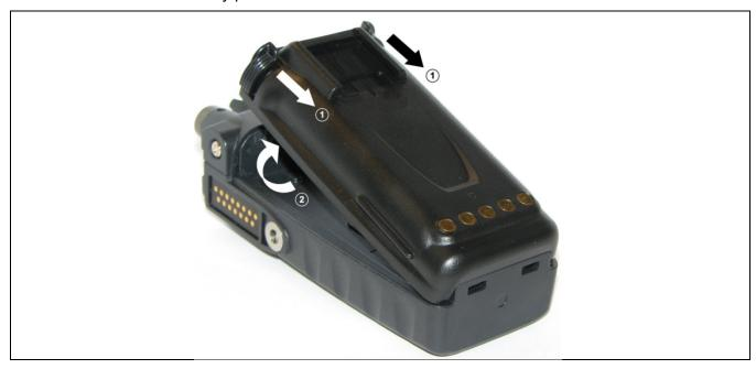
Figure 3-2: Remove the Battery
