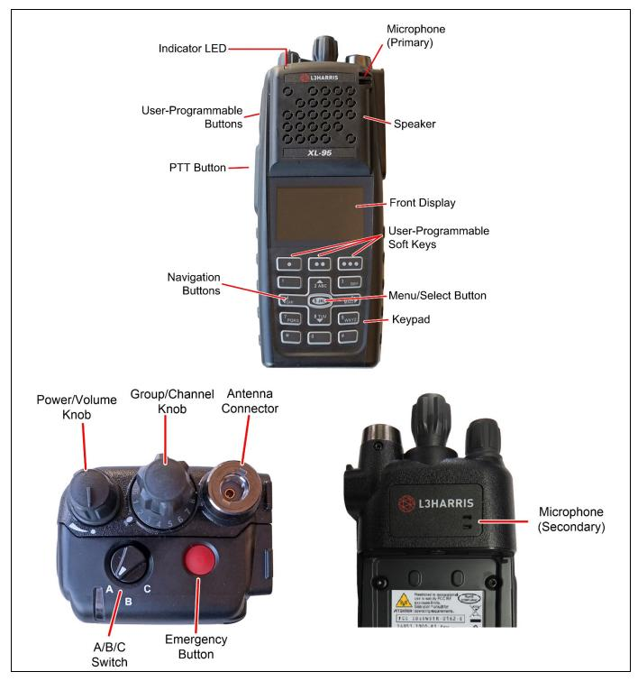
Figure 4-1: Radio Controls, Indicators, and Connectors
