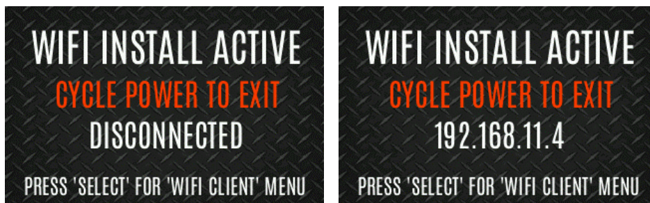
Figure 12-5: Enable Wi-Fi Programming Mode on Radio
