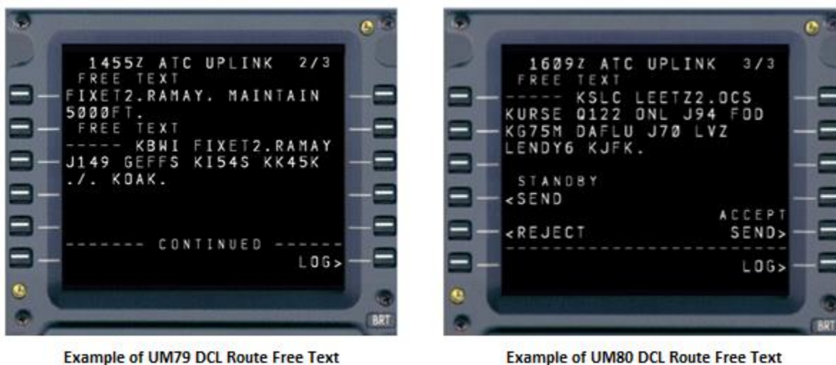
Figure 1 – CPDLC Departure Clearance with Route Free Text
