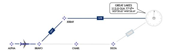
In the figure above, ATC sends the clearance CLEARED TO [GLA] VIA [BRAVO Q97 XXRAY Q38] to the aircraft using CLEARED TO [position] VIA [route clearance]. There is no discontinuity at BRAVO because the uplink fix [BRAVO] is in the existing cleared, active flight plan loaded in the FMS.
