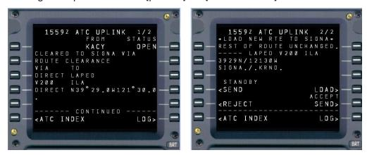
This capability is a powerful feature of En Route CPDLC in the U.S. NAS. However, its benefit is only realized if flight crews use the LOAD or INSERT (i.e., "Push-to-Load") functionality of the FMS. <u>Do not attempt to build these revised route clearances in the FMS on your own. Use the LOAD or INSERT function.</u>
