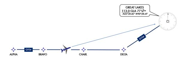
Note: If a LOAD prompt is available, it should be used. Not all aircraft have the capability to load information from CPDLC message into the FMS e.g., PROCEED DIRECT TO RBV may not be loadable on one airframe where it is loadable on others. See aircraft documentation for additional information.
