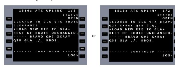
Note: Some systems may display only the message "CLEARED TO [position] VIA ROUTE CLEARANCE" and the pilot must load the route into the FMS to see/verify the modified route or reclearance via their Nav Display. Other aircraft may display the actual uplinked route received from ATC. FAA's Route Verification Text is intended to help resolve any ambiguity.
