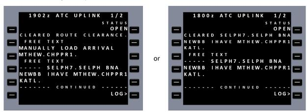
Note: Some systems may display only the message "CLEARED ROUTE CLEARANCE" and the pilot must load the route into the FMS to see/verify the new/modified route clearance on the nav display. Other aircraft may display the actual uplinked route received from ATC. FREE TEXT is intended to help resolve any ambiguity.
