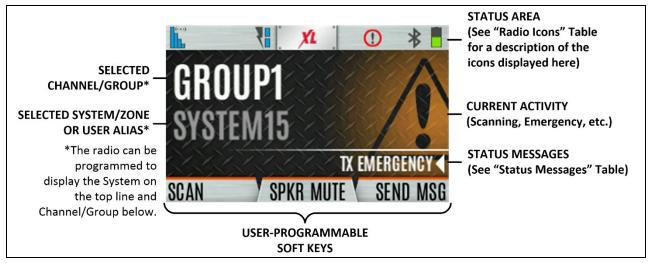
Figure 5-4: Sample Idle Front Display
