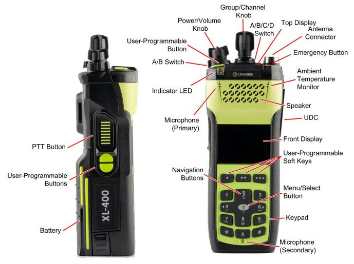
Figure 5-1: Radio Controls
