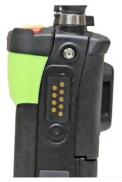
Figure 4-3: Universal Device Connector
