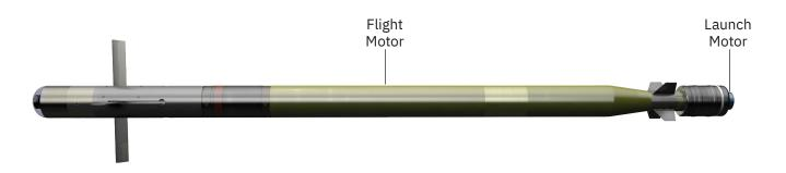
The Raytheon-produced Stinger missile is launched by a small launch motor that pushes it a safe distance from the operator before engaging the main flight motor. Aerojet Rocketdyne provides both solid propellant rocket motors.
