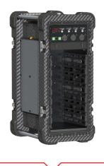
The L3Harris DTOK (12006-2200-01) is the larger next-generation modular box. The scalable platform allows for a large variety of C5ISR solutions including: LOS, SATCOM, mobile ADHOC networking (MANET), and the ability to integrate with existing networking infrastructures and equipment. The DTOK can be used in tactical operation centers (TOC), aircraft, and vehicles.
