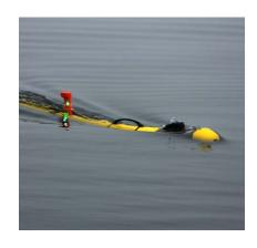
The Iver4 580 is the second vehicle in the Iver4 family of next-generation AUVs. It offers users a 300-meter depth-rated survey system featuring six-hour endurance hot-swappable sealed battery sections that can be quickly changed in the field, allowing for quick turn-around times with no realignment of the INS or vacuum required.
