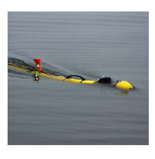
The Iver4 580 is the second vehicle in the Iver4 family of next-generation AUVs. It offers users a 300-meter depth-rated survey system featuring six-hour endurance hot-swappable sealed battery sections that can be quickly changed in the field, allowing for quick turn-around times with no realignment of the INS or vacuum required.
