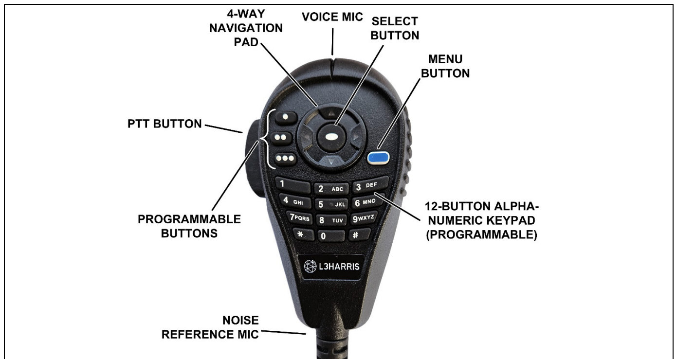
Figure 4-2: Keypad Mobile Microphone (KMM) Controls
