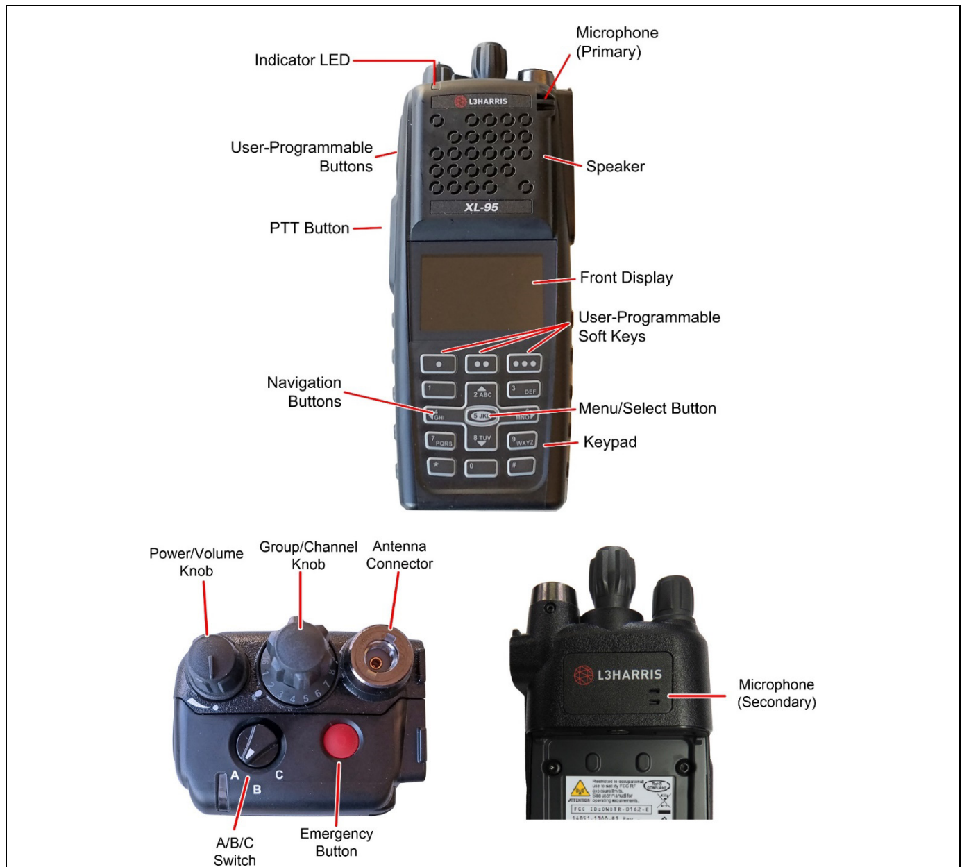
Figure 4-1: Radio Controls, Indicators, and Connectors
