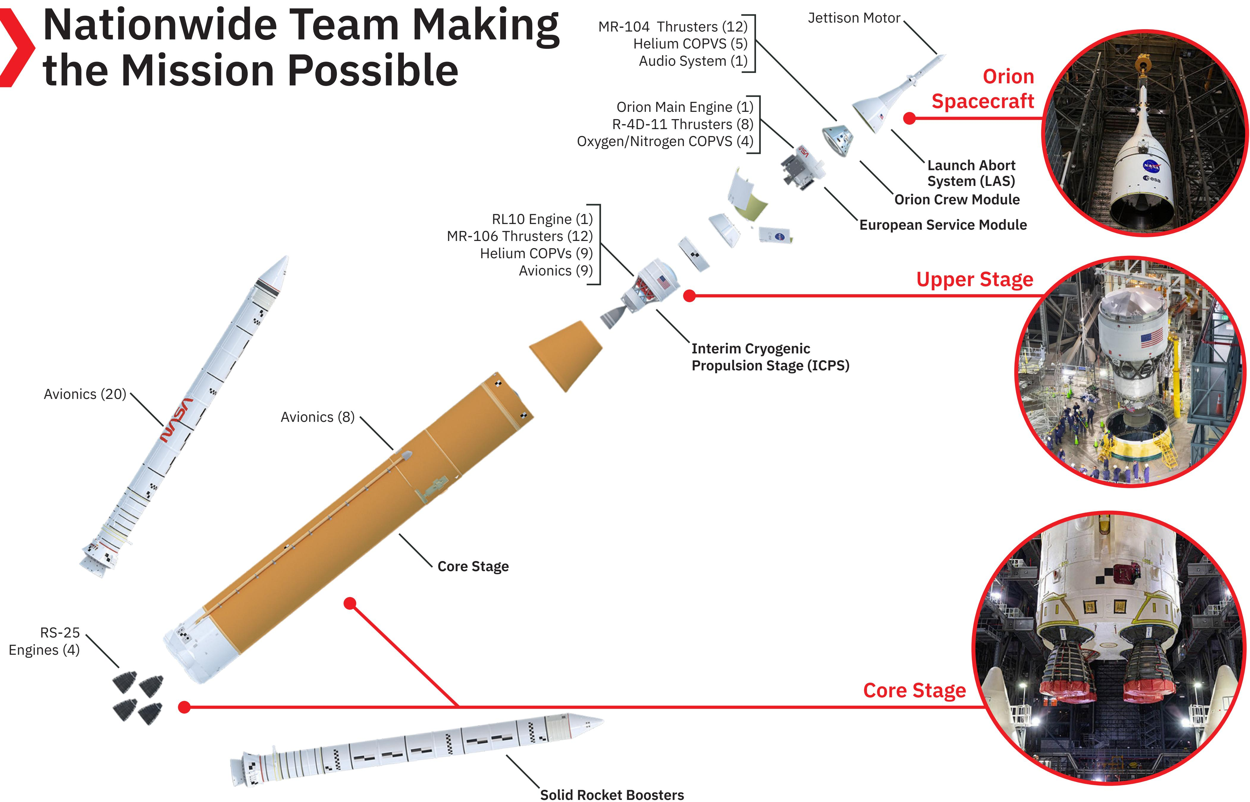
L3HARRIS HAS 103 ELEMENTS ON THE ARTEMIS II ROCKET, INCLUDING EQUIPPING EACH ASTRONAUT WITH TWO SMALL OXYGEN TANKS THAT CAN BE USED IF AN EMERGENCY ARISES
