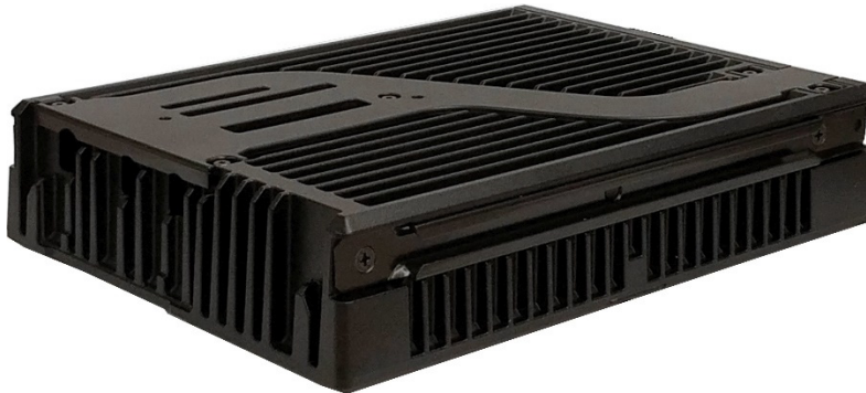
Figure 3-1: Vehicle Communications Hub (VCH)
