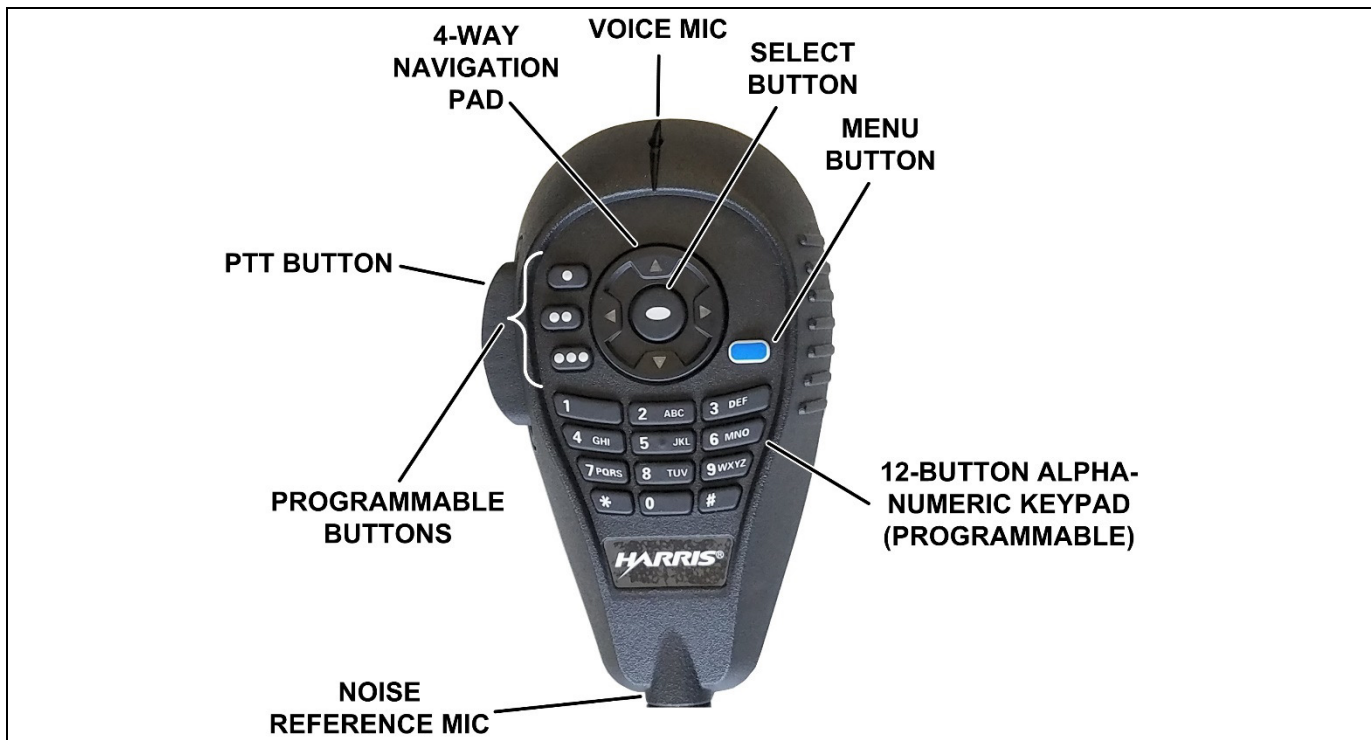
Figure 4-2: Keypad Mobile Microphone (KMM) Controls
