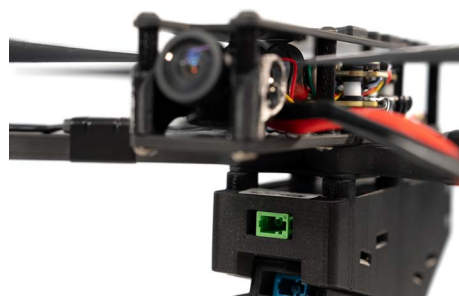
Far-end unit w/ LC-APC connector
