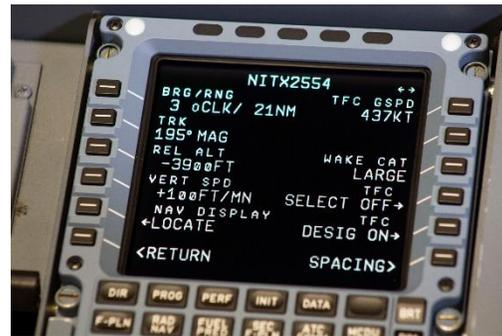
The **CDTI Assisted Visual Separation (CAVS)** application aids flight crew in managing spacing that is more efficient during final approach during challenging visual conditions. The CAVS application has shown to reduce aircraft final approach time by as much as 14% in marginal weather, can help reduce go-arounds and can help keep flights running on time during reduced visibility conditions.
